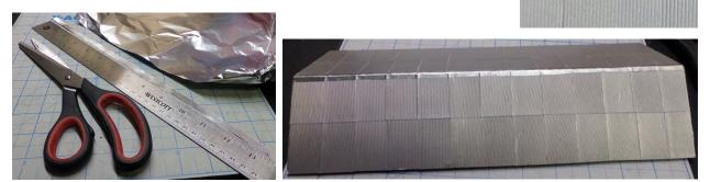
These 2 above images are showing how to make the aluminum foil ¼" wide strip. We use the back side facing up. Now add glue along the roof top center and press the aluminum foil strip in place. Trim the ends.
