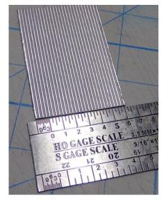
All these adhesive backing metal siding strips must be cut to scale width. These were cut to 7 scale feet width to allow any alignment trimming needed later on. Below I made a jig to cut from top to bottom with a Exacto Knife. Start at the bottom corner and slightly overlay the next side adjoining panel till the bottom row is complete.
