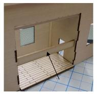
Next the extension walls and floor are assembled. Glue the top cross brace, floor and the 2 back corner braces. (1/8 X 1/8 X 2 3/8") Do not glue the wide center brace, this holds it open as it is glued to the wall opening. Once the glue has cured a few hours, remove the wide brace.
